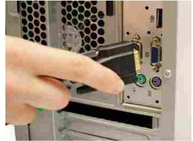
Connecting the monitor cable to the VGA port
