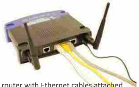
A router with Ethernet cables attached
